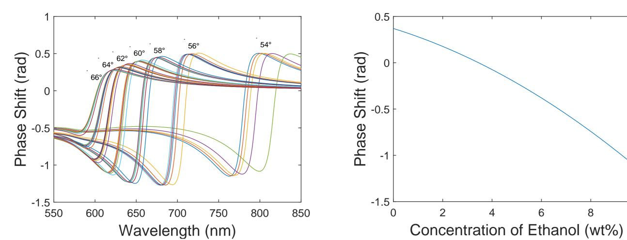
Figure 2: Theoretical phase shifts computed for several angles of incidence and five analytes with various wt% of ethanol.
