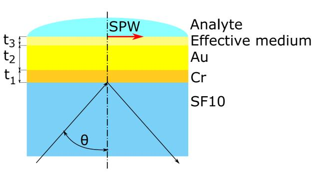
Figure 1: The SPR structure considered for theoretical modeling.
