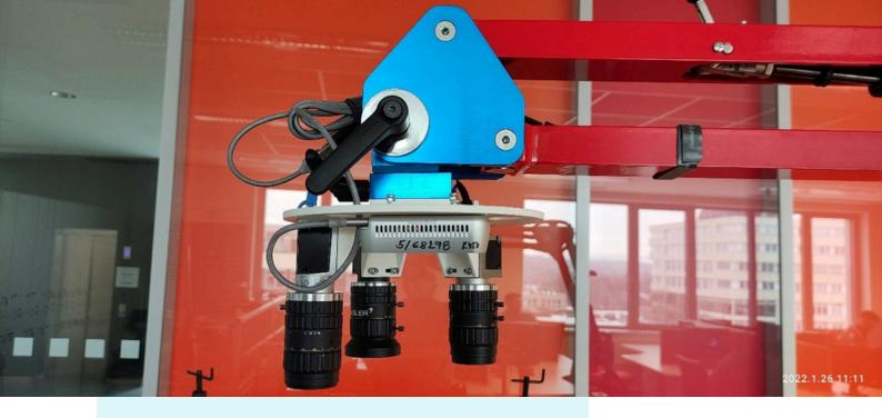
The research project of a complex test equipment for product's total quality control (TQC) with the implementation of machine vision algorithms in robotics technology for the automated process of camera composition based on input data in the form of a 3D product model and precise specification of the controlled area. The results of the research help automate and significantly accelerate the development of industrial applications with camera inspection.
