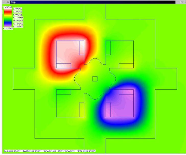
Figure 7.10: Magnetic flux lines for the *diagonal current excitation* ( $v := 2$ ) for the Maltese Cross
