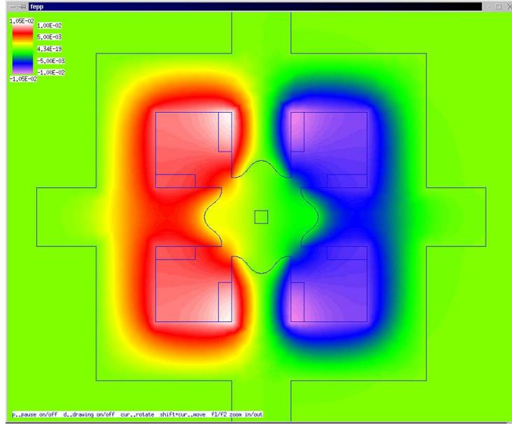
Figure 7.9: Magnetic flux lines for the *vertical current excitation* ( $v := 1$ ) for the Maltese Cross
