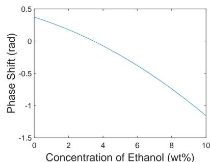
Figure 3: Phase shift as function of concentration of ethanol in analyte ( $\lambda = 700.91$  nm, angle of incidence  $56^\circ$ ).
