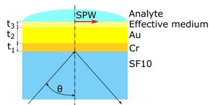
Figure 1: The SPR structure considered for theoretical modeling.
