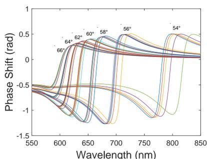
Figure 2: Theoretical phase shifts computed for several angles of incidence and five analytes with various wt% of ethanol.
