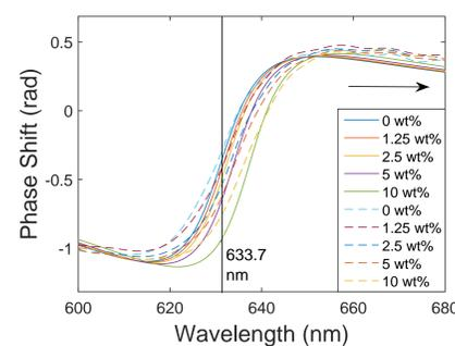
Figure 8: Phase shifts - comparison of the theory and experiment.
