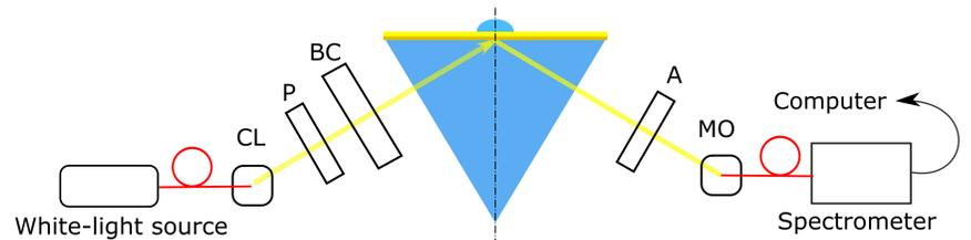
Figure 6: Experimental setup consisting of white-light source, collimating lens (CL), polarizer (P), birefringent crystal (BC), analyzer (A) and microscope objective (MO), spectrometer and computer.
