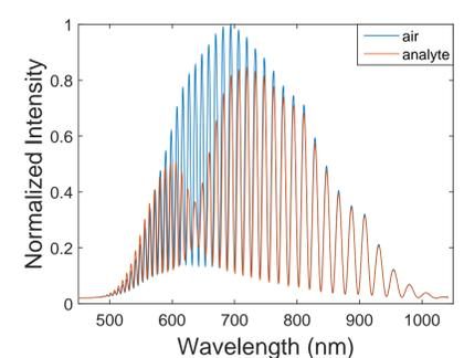
Figure 7: Two channeled spectra and one with visibility decrease. Concentration of ethanol is 10 wt%.
