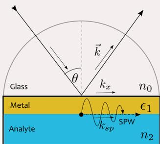
Schematic configuration of a system exciting surface plasmon wave (SPW)
