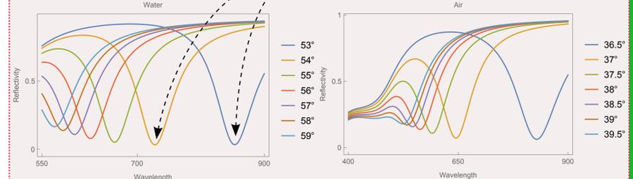
Reflectivity for different angles of incidence and thickness 35 nm.
