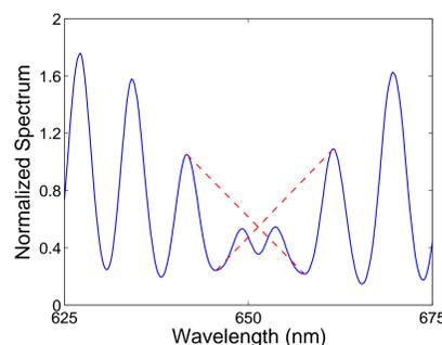
**Figure 6:** Recorded normalized spectrum with lines enabling determination of the wavelength of the envelope minimum.
