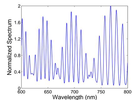
**Figure 5:** Recorded normalized spectrum corresponding to mirror displacement  $\Delta l_2 = 101 \text{ nm}$ .
