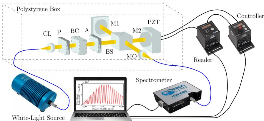
**Figure 1:** Experimental setup with a Michelson interferometer to measure mirror displacement; collimating lens (CL), polarizer (P), birefringent crystal (BC), analyzer (A), beam splitter (BS), mirrors (M1, M2), piezo transducer (PZT) and microscope objective (MO).
