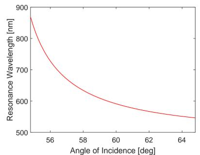
Figure 6: Resonance wavelength as a function of the angle of incidence on the dielectric-metal boundary (ethanol).
