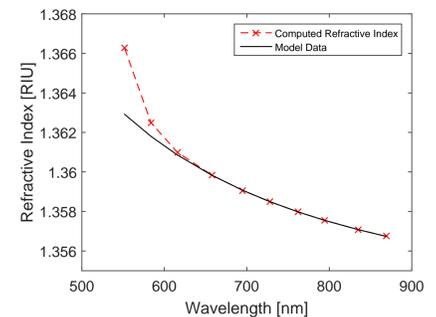
Figure 8: Refractive index of ethanol as a function of wavelength (the first procedure).
