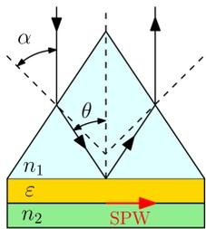
Figure 1: The schematic drawing of the Kretschmann configuration with an equilateral coupling prism.
