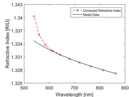
Figure 7: Refractive index of water as a function of wavelength (the first procedure).
