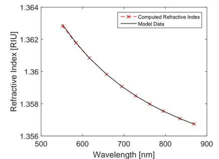
Figure 10: Refractive index of ethanol as a function of wavelength (the second procedure).
