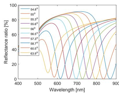
Figure 4: Theoretical spectral dependencies of the reflectance ratio  $R_p(\lambda)/R_s(\lambda)$  for different angles of incidence (ethanol).
