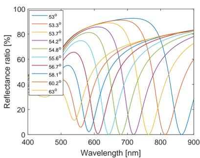
Figure 3: Theoretical spectral dependencies of the reflectance ratio  $R_p(\lambda)/R_s(\lambda)$  for different angles of incidence (water).
