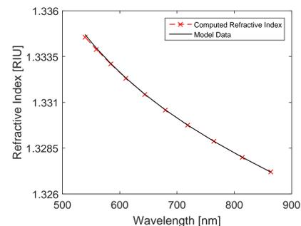
Figure 9: Refractive index of water as a function of wavelength (the second procedure).
