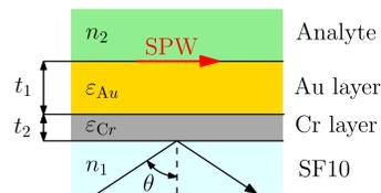
Figure 2: The schematic drawing of four-layer SPR structure used in theoretical model.
