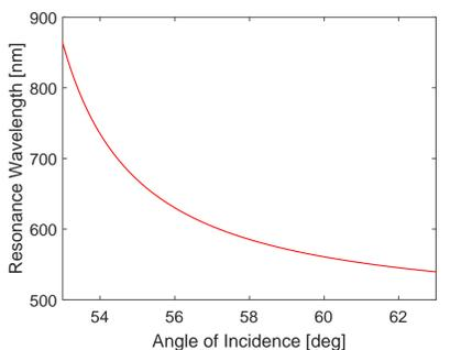
Figure 5: Resonance wavelength as a function of the angle of incidence on the dielectric-metal boundary (water).
