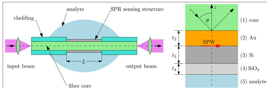
Figure 1: The crosssection of fiber optic sensor part and equivalent five-layer structure
