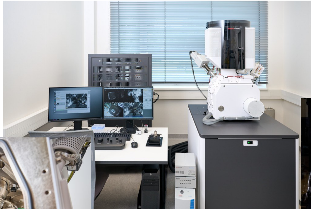
High Resolution Scanning Electron Microscope combined with X-ray Photoelectron Spectroscopy (HRSEM/XPS)
